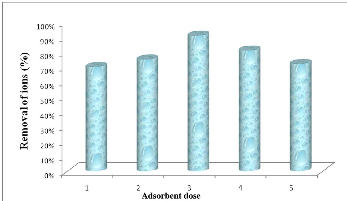
**Figure 4:** Variations of % removal of Pb by adsorbent dose in 120 min. as contact time and pH 5
