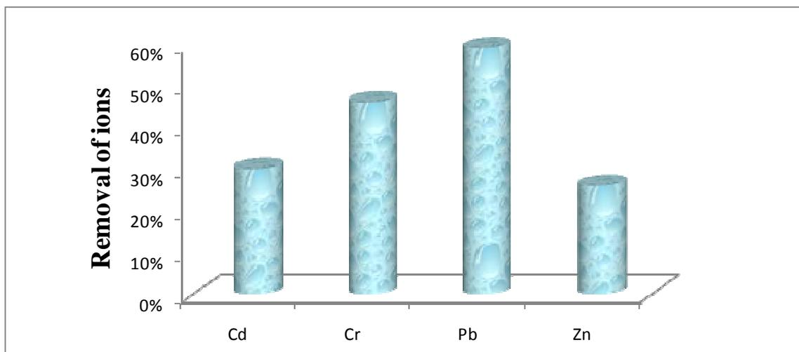
**Figure 1:** Biosorption (removal %) of metal ions (Cd, Cr, Pb and Zn) by dried water hyacinth leaves (1 gm) at pH 7 and contact time 1 hr.
