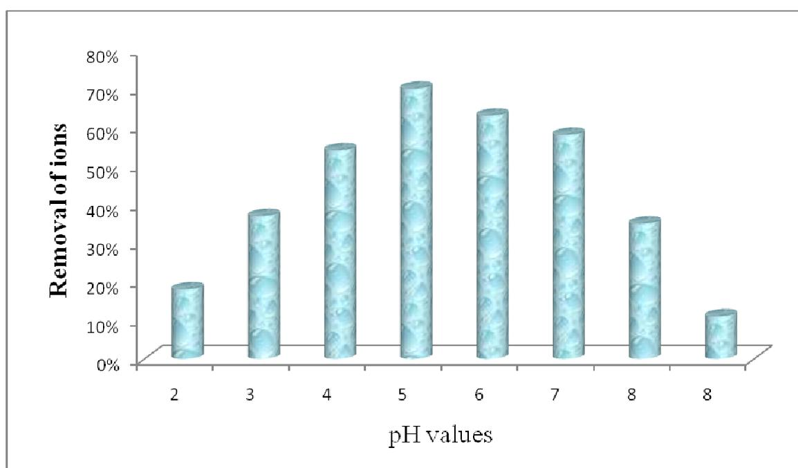
**Figure 2:** Effect of pH on removal of Pb by 1 gm of dried water hyacinth leaves at contact time 1 hr.
