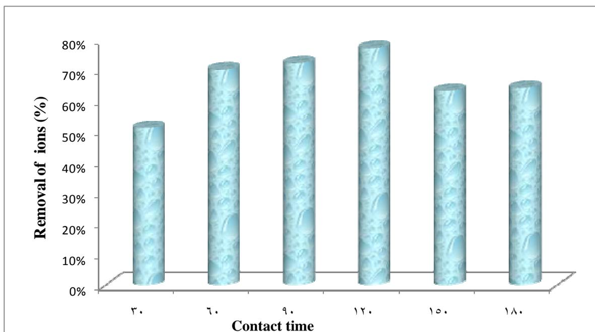
**Figure 3:** Effect of contact time on removal of Pb by 1 gm. of dried leaves of water hyacinth at pH 5
