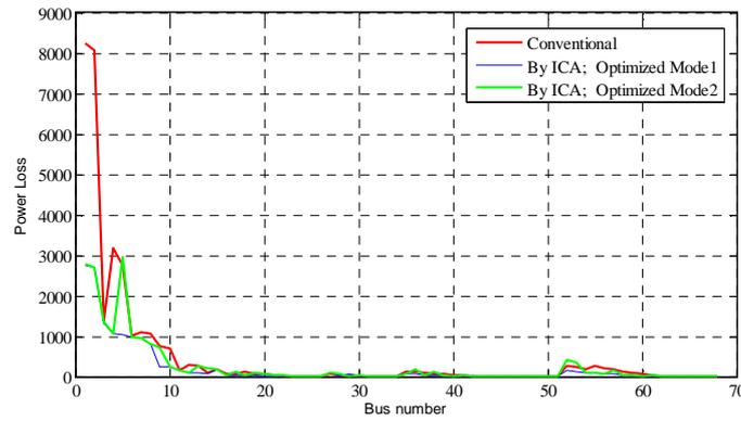
**Fig 5:** Peak power loss profiles in each branch
