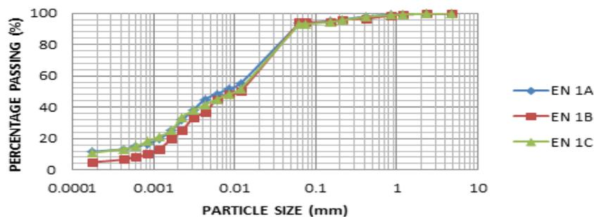
**Figure 2:** Grading curves of Ugbo-Odogu shales
