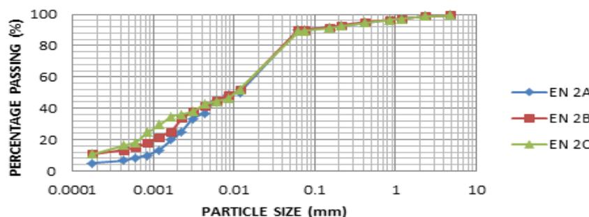
**Figure 3:** Grading curves of Gariki shales
