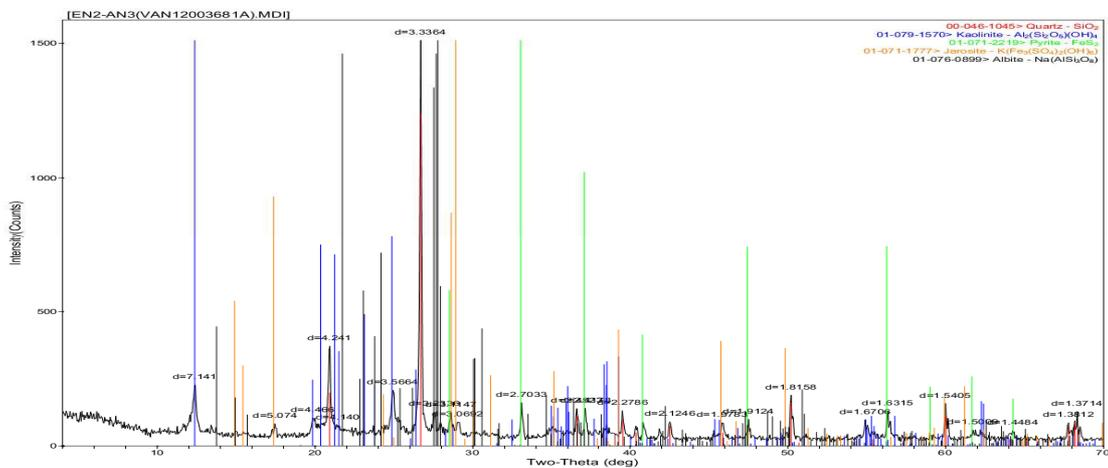
**Figure 6:** Diffractogram of Gariki shale
