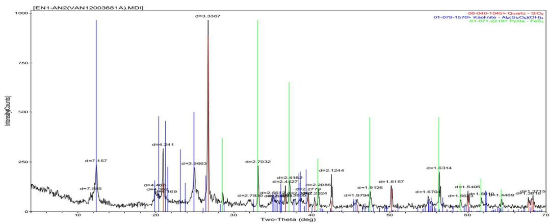
**Figure 5:** Diffractogram of Ugbo-Odogu shale
